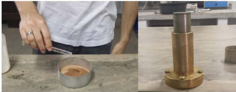
Figure 6: Static compaction at a specified moisture content and density
