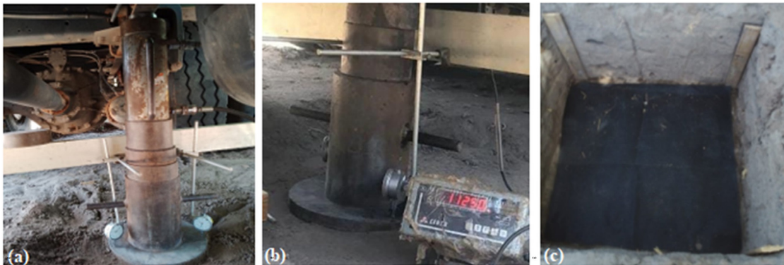
Figure 5. Load tests: (a) natural soil; (b) compacted soil; (c) compacted soil with microgrid.
