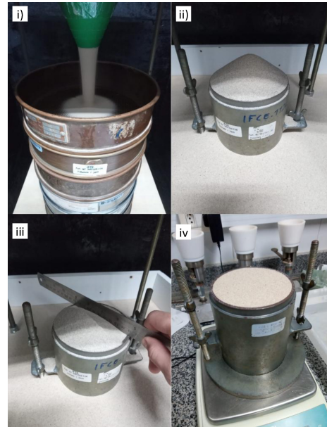
(b) Stages of the pluviation procedure. i) pluviation process; ii) pluviated material; iii) surface leveling; iv) weighing of the set.
